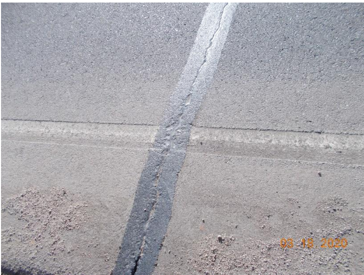
Suspect asbestos-containing material I-13-H-TR01. The tar material is non-detect for asbestos.
